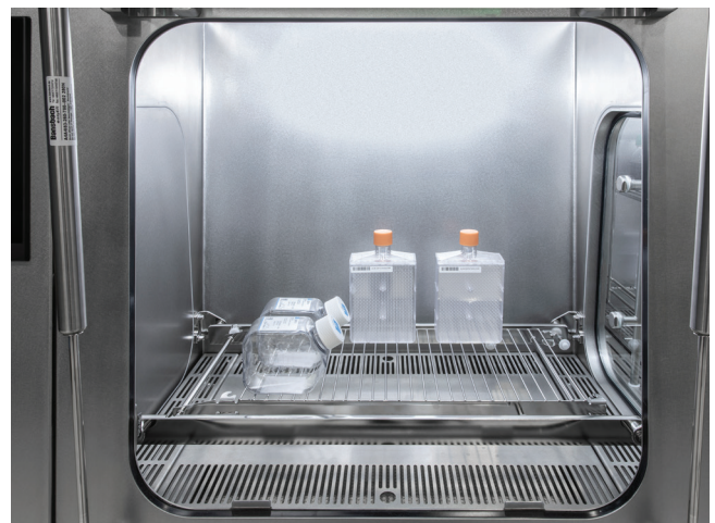
Safe and rapid transfer airlock (SARA)
