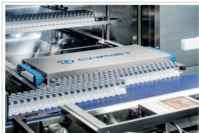
Figure 3. Advanced loading and unloading system for a GMP-freeze dryer.
