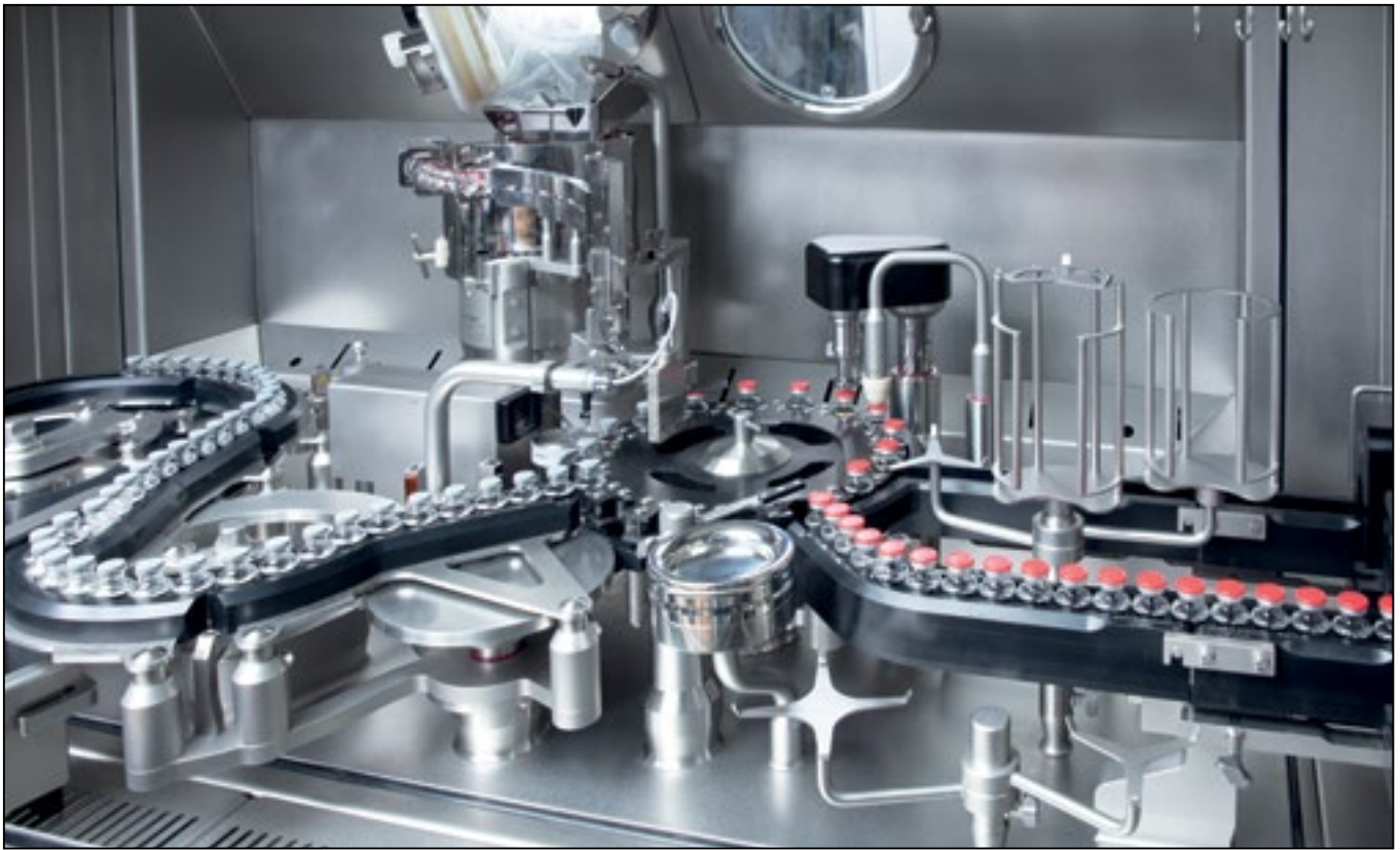
Fully automatic closing vials
