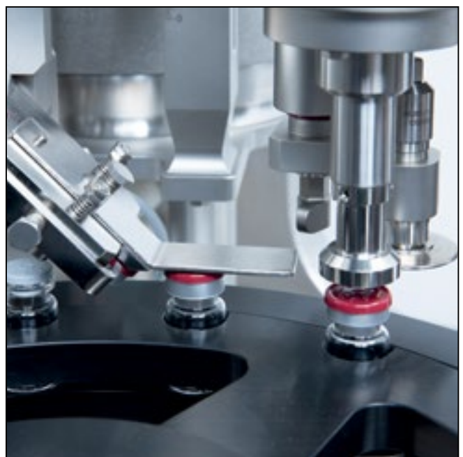
Closing station for crimp caps
