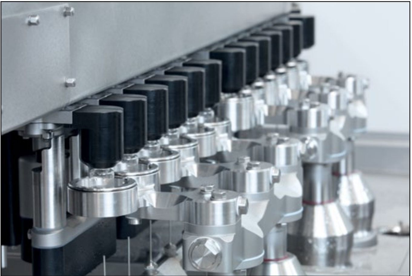
360° cleaning thanks to special ring jets
