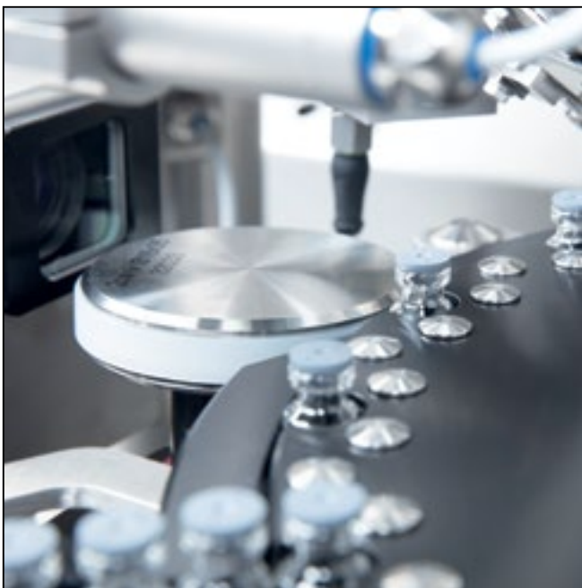
Stopper gap detection
