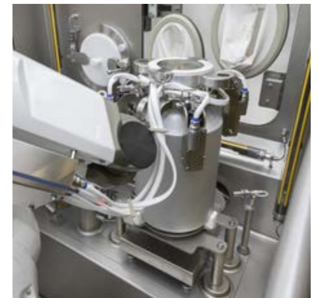
Robotic handling and transfer of a potent powder in an aseptic isolator.
