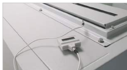
Measuring the Temperature of the Air Outflow
