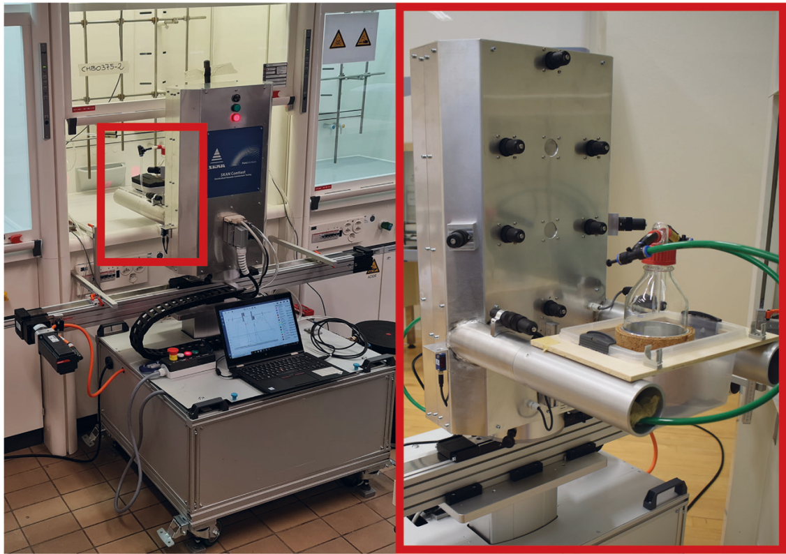
Figure 1. A Contest test setup under field conditions (photograph by courtesy of EPFL, CH-Lausanne), at left. View on front side of the body with sensors (black cartridges on the body), arms, and vaporizing bottle, at right.
